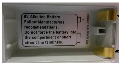
Battery compartment connectors in correct position
