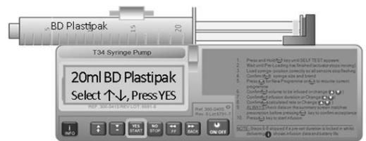
Either use a compatible syringe brand or arrange for the new type of syringe brand to be configured into the pump by authorised personnel.
