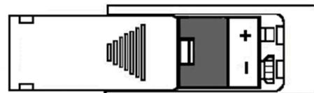
2. Push the battery into the compartment taking care to ensure that the battery + / - contacts are aligned on the label inside the compartment.
