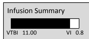
The syringe volume to be infused (VTBI) and volume infused (VI) display. (The total of the two values equal the starting volume).
